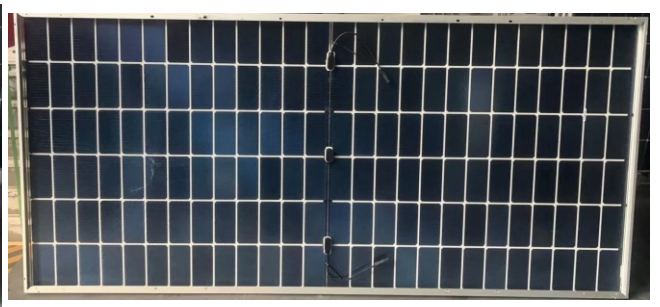
Sample #1-fire 6: Burning brand test (back)
